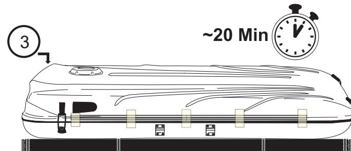
**EN** Apply adhesive tape to help fixating the profile while the glue reacts. In case of glue spilling, clean as soon as possible as it may damage the tent coating.
