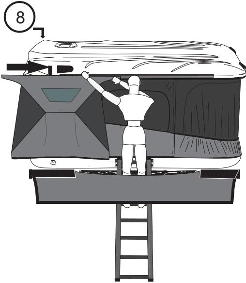
**EN** Slide the cable into the black plastic profile, and center the tunnel with the tent door.
